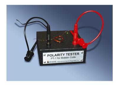
The PT-1 provides a simple and easy way to determine the relative polarity of bobbin coil windings. By placing a coil on the platform and making connection to the start and end of a winding, a test signal is induced in the winding. Depending on the direction of the winding, a Red / Green LED will indicate the relative polarity. The induced signal is very low level and completely safe to the operator.
